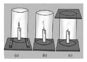
From the above three experimental setups we can see that the candle burns freely when there was a continuous supply of air as in the first case. The candle started flickering when we had stopped the air supply from the bottom as in the second case. Finally in the third case when we had removed the supply of air from both the bottom and above the candle goes off.
